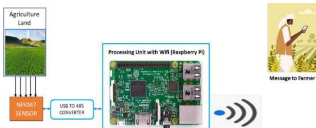
Figure 1. Block diagram of the proposed IoT based fertilizer notification system
