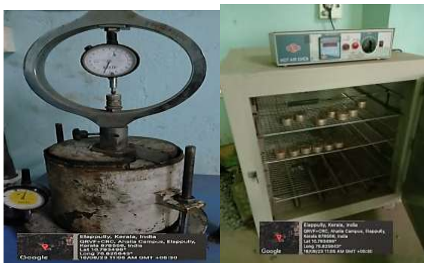
Figure 9: California Bearing Ratio Test on BCS.
