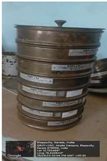
Figure 6: Sieve Analysis on Black Cotton Soil.
