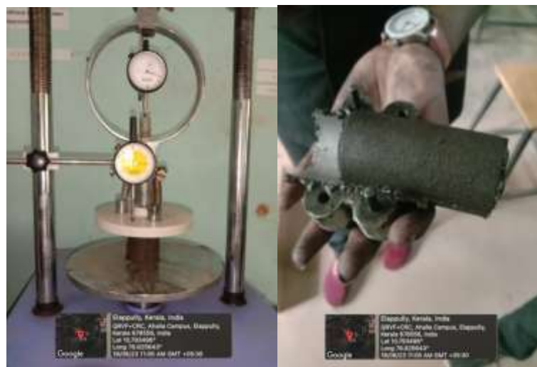
Figure 01: Unconfined Compressive Strength Test on BCS.
