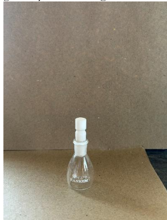
Fig 8: Relative density bottle
