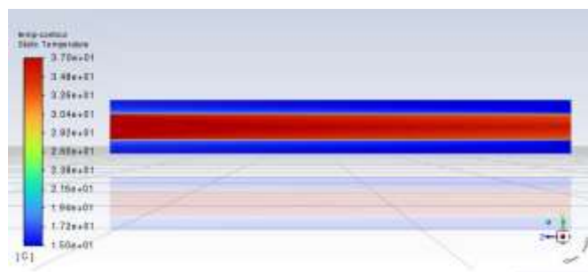
Figure 3. Temperature Distribution of cardioplegia concentric tube heat exchanger
