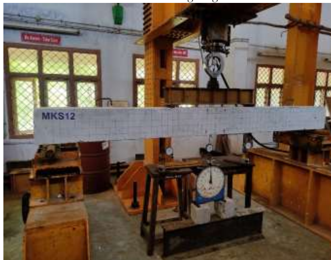
Fig 6 Static Test Set-up
