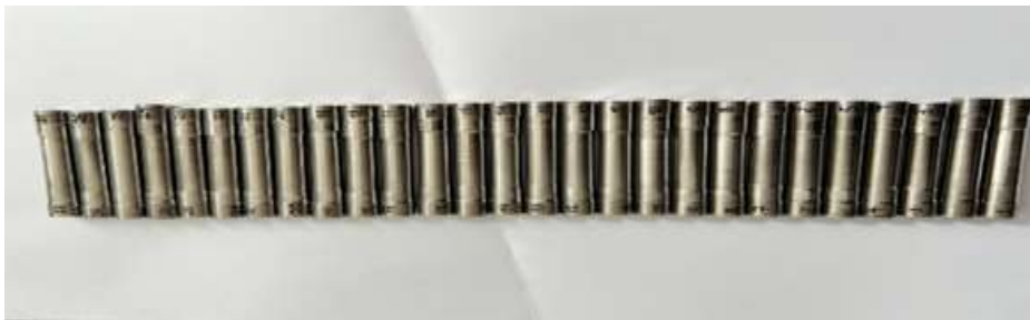
FIGURE 1. Machined tensile samples with a cutting length of 70 mm and a diameter of 9 mm
