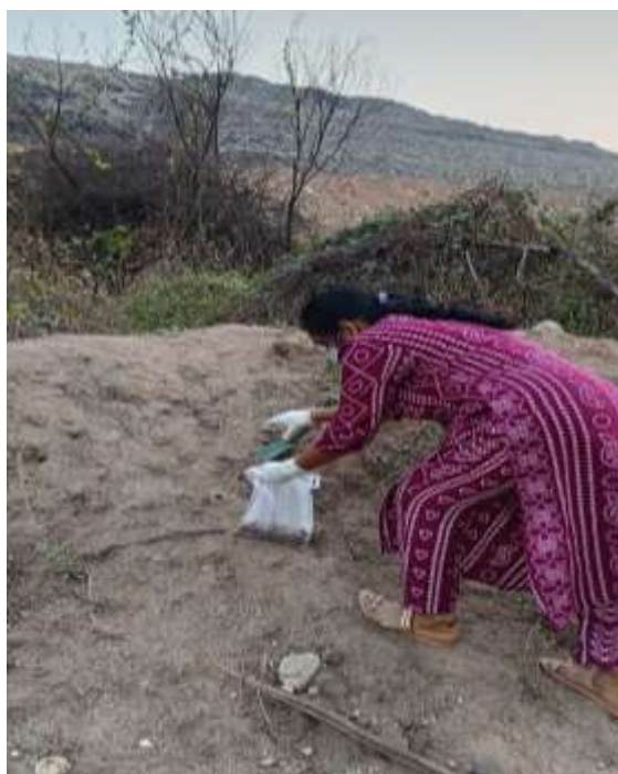
Figure 4: Field sampling near the landfill using a trowel and labelled HDPE bags.
