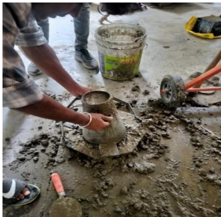
Figure:6 Slump Test.
