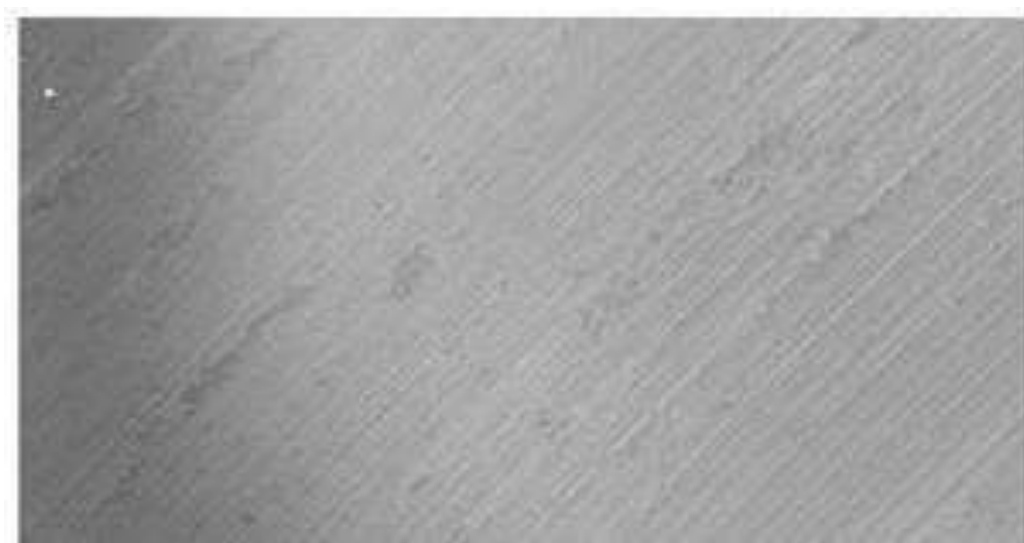
Fig. 5.11 SEM micrograph of worn surface of Al6061+WC-2%+fly ash-6% at 4.91N normal load and sliding velocity 1m/s.
