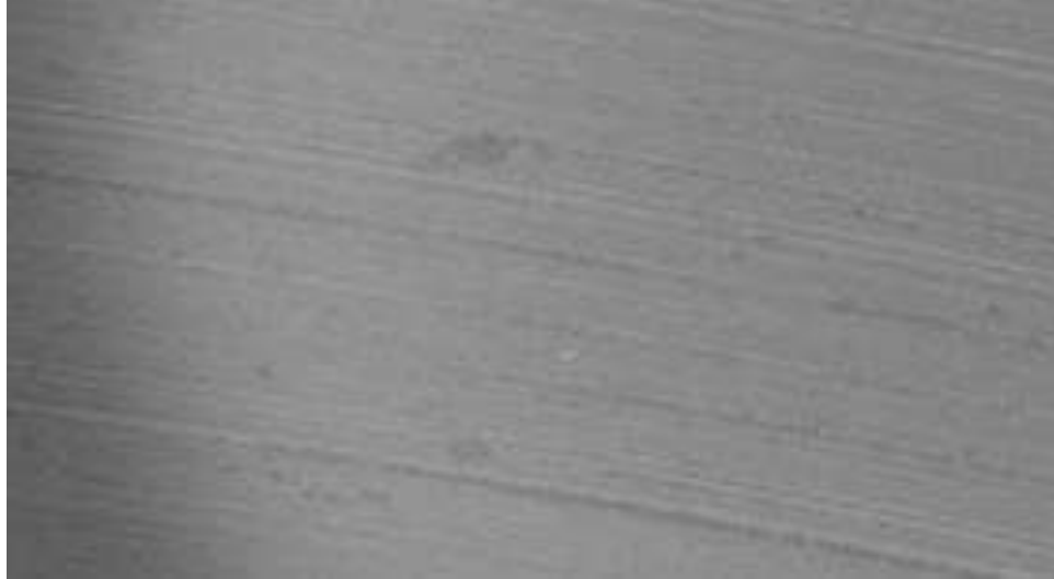
Fig. 5.12 SEM micrograph worn surface of Al6061+WC-2%+fly ash-6% at 9.81N normal load and sliding velocity 1m/s.
