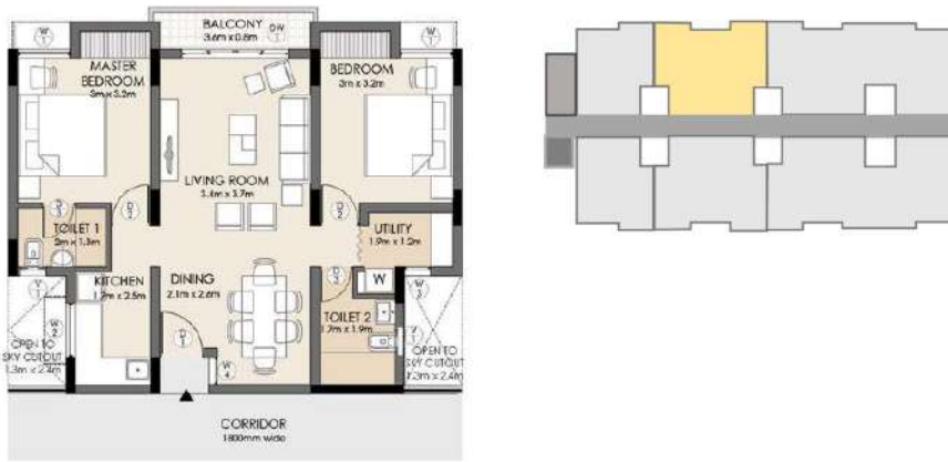
Figure 6: Selected unit and block typology from “Handbook of replicable design for energy-efficient residential buildings” by BEE, Ministry of power, Government of India (Unit size - 65 Sqm, 2 BHK, Appropriate for mid rise)
