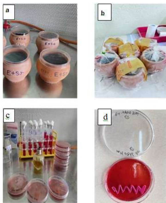
Figure 4: Experimental setup and microbial analysis: (a) Prepared mud pots with and without Fe-TiO 2 coating; (b) Autoclaving of pots before experimentation; (c) Preparation for MPN method and streaking onto petri dishes (d) Showing bacterial growth without coating of Fe-TiO 2 on one side and no growth in Fe-TiO 2 on the other side at 7 hours, done by the MPN method.
