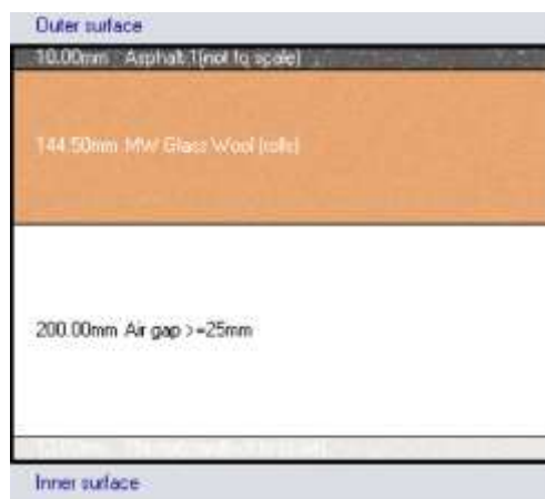
Fig.12 Roof detail from Design Builder
