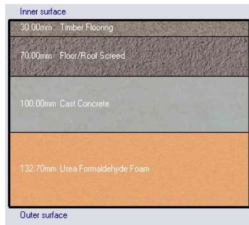
Fig.26 Roof detail from Design Builder
