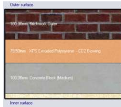
Fig.5 External wall detail from Design Builder
