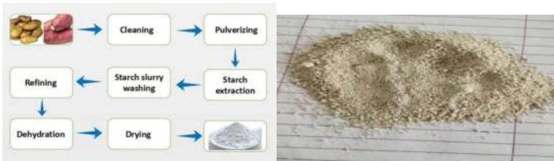
Figure 2: Conventional method for extraction of starch from purple yam
