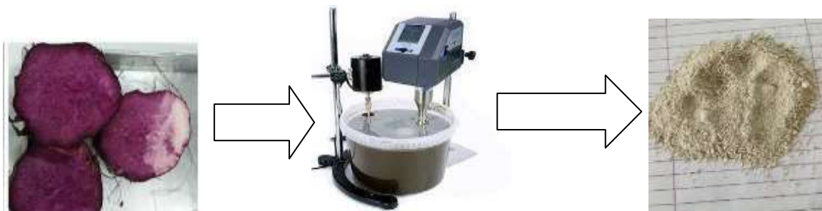
Figure 3: Ultrasound method for extraction of starch from purple yam
