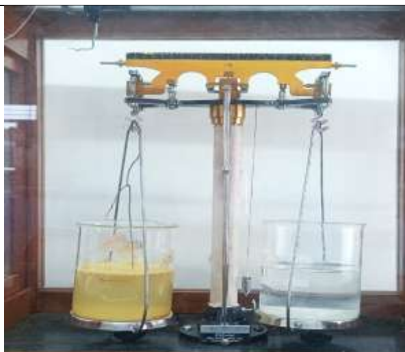
Figure.5:Modified apparatus for raft strength measurement
