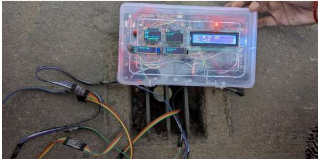
Fig.16. Real-time vibration monitoring setup deployed on the Bhakta Kannappa Sethu Bridge using a microcontroller-enabled MEMS accelerometer system.
