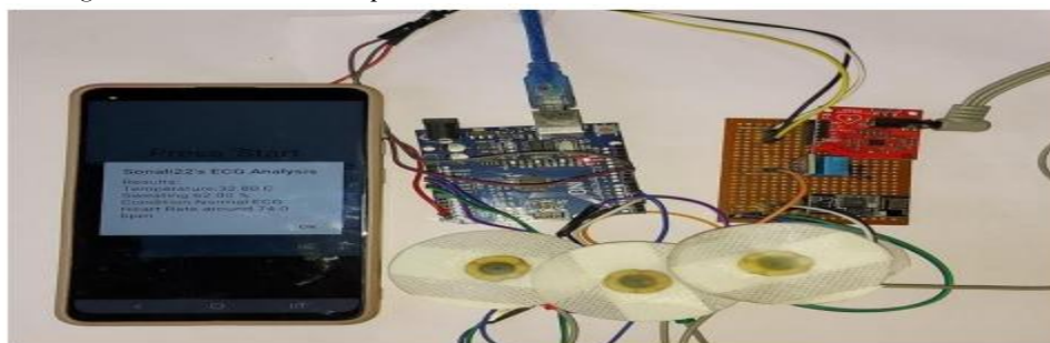
Figure 2: Hardware Setup of IoT-Based Wearable Device for ECG Monitoring
