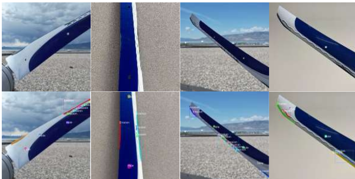
defect detection, the dataset was filtered to include only the 3,000 images with visible damage. Fig. 1 Samples from the dataset captured at UVU with the raw images (top) and annotated images (bottom).
