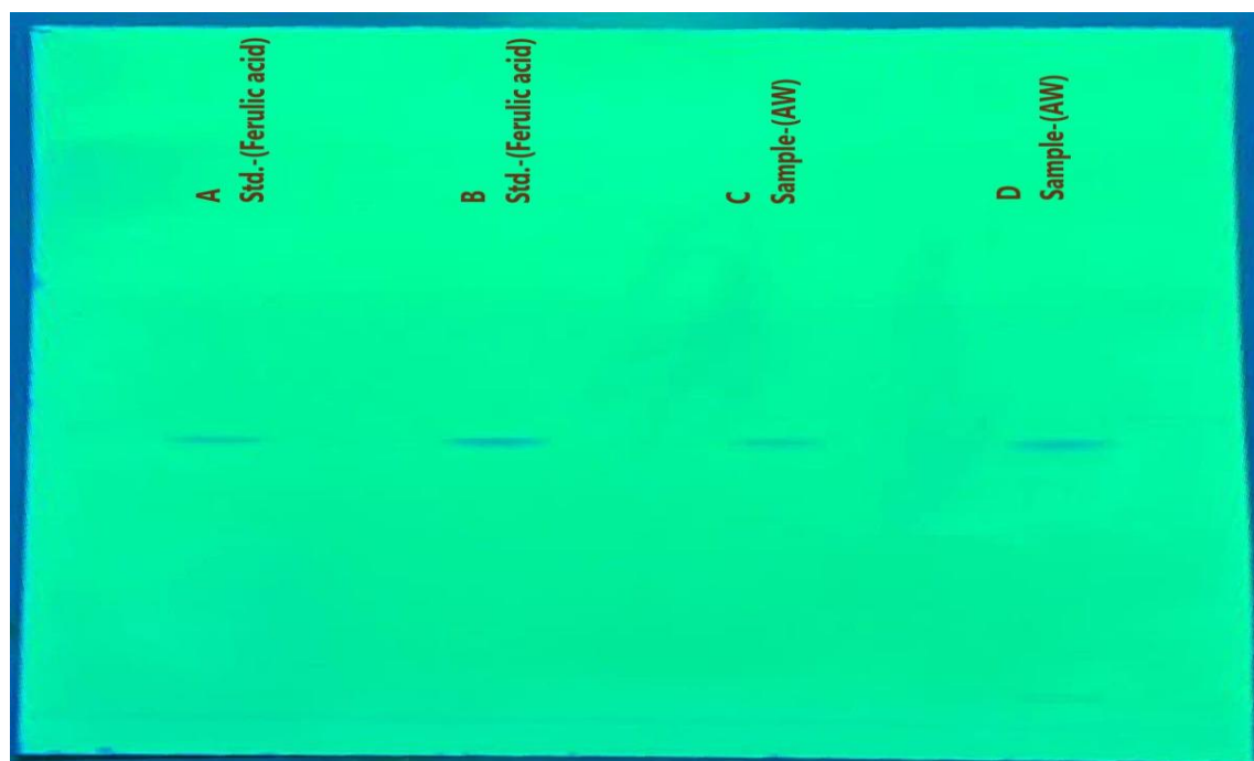
Figure 1: Chromatogram obtained from separation of AW Sample and visualized under UV light of wavelength 254 nm
