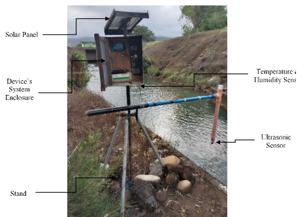
Fig. 4. Automated Water Level and Discharge Measuring Device
