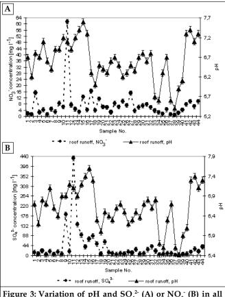
Figure 3: Variation of pH and SO<sub>4</sub><sup>2-</sup> (A) or NO<sub>3</sub><sup>-</sup> (B) in all Roof Runoff Samples
