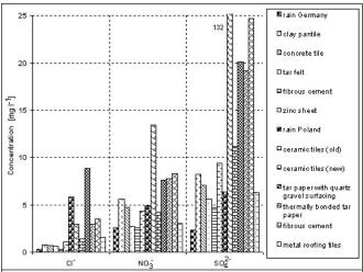
Figure 2: Comparison of Anion Concentration in Rain and Roof Runoff Samples from Selected Roof Coverings
