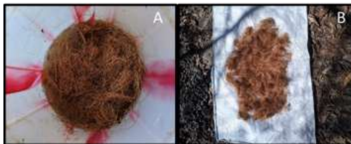
Figure 3: Coir fibre (A) soaked in oil (B) dried under the sun
