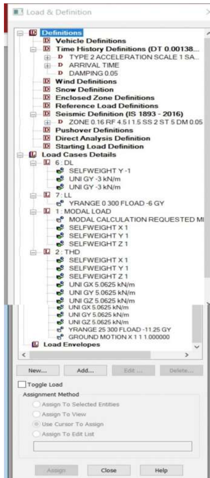
Fig: 5 Shows the loads applied
