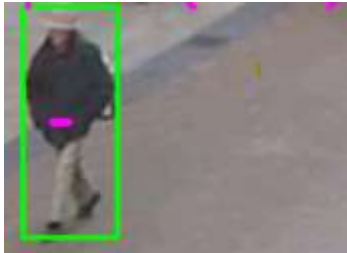
Fig. 2. Detection results of motion target tracking using the Kalman filter.
