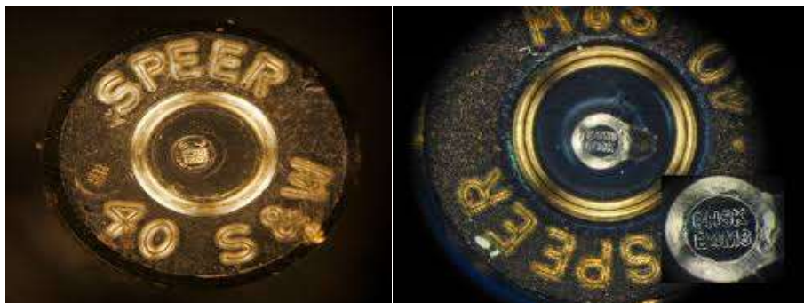
Figure 4 and 5: Cartridge cases showing microstamped identification codes [4].
