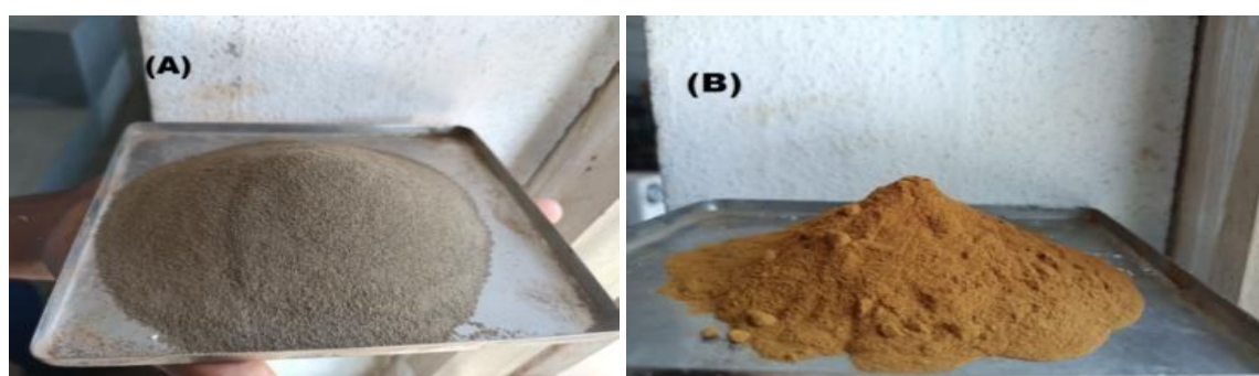
Figure 1: (A) Black cotton soil (B) Calcium lignosulfonate
