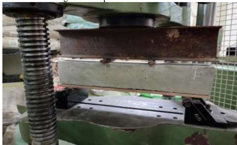
Figure 2. Four-Point Bending Test Setup for Crack Induction in Fibre-Reinforced Concrete Beam Result and Discussion
