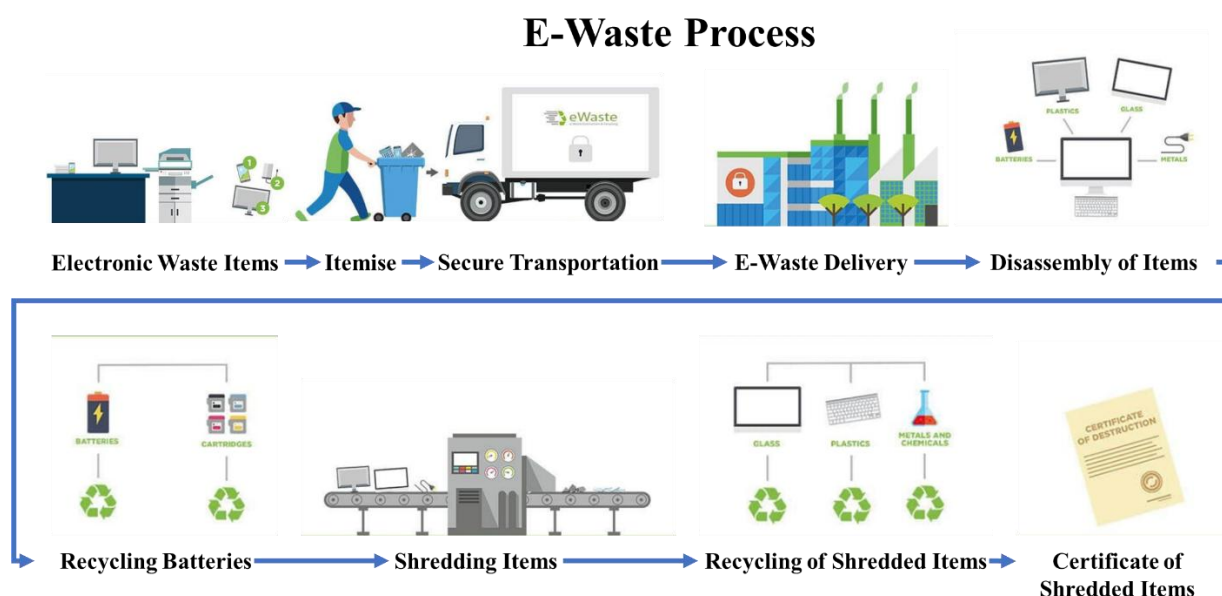
Figure 4. Process of EWM System.
