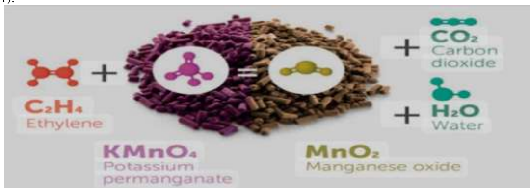
Fig. 1 : Ethylene molecules reacting with KMnO 4 giving CO 2 and H 2 O.
