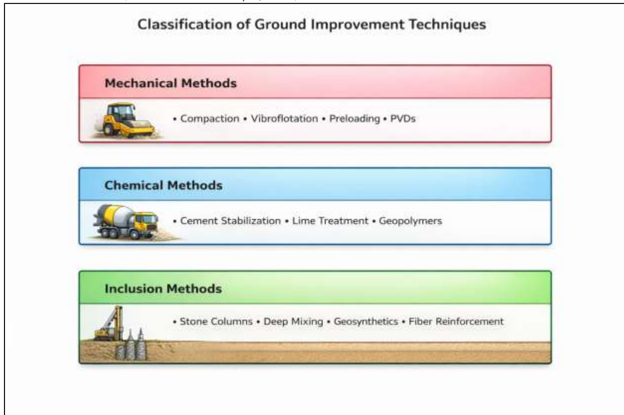
Figure 3 Classification of Ground Improvement Techniques
