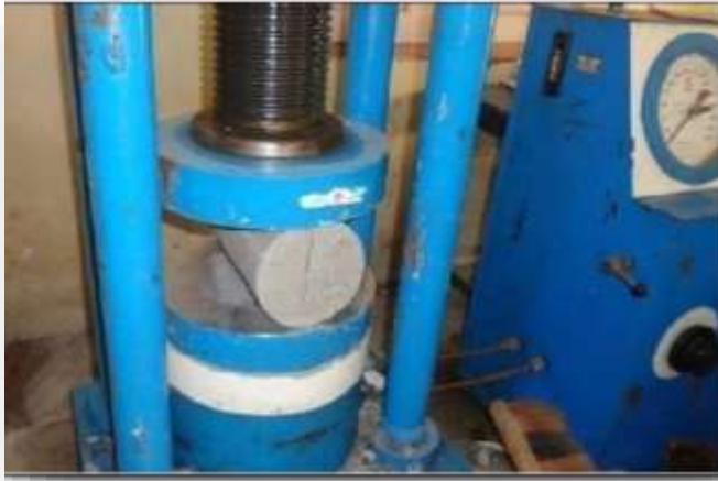
Fig 2. Split tensile strength test carried out on cylinder specimen in Compression testing machine
