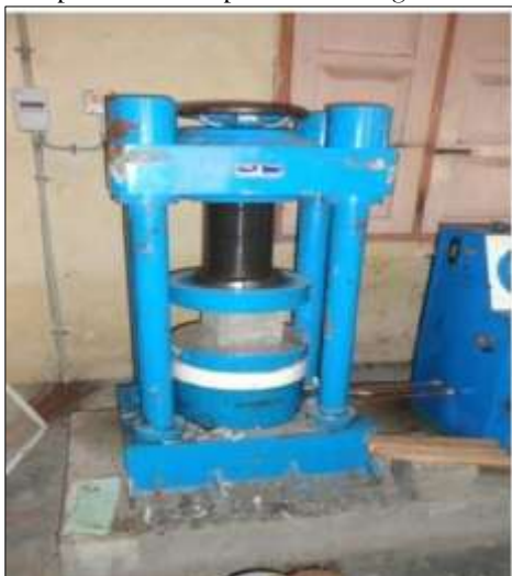
Fig 1. Compression test carried out on cube specimen in Compression testing machine
