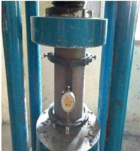
Fig 4. Cylinder specimen positioned with test setup for Young modulus test
