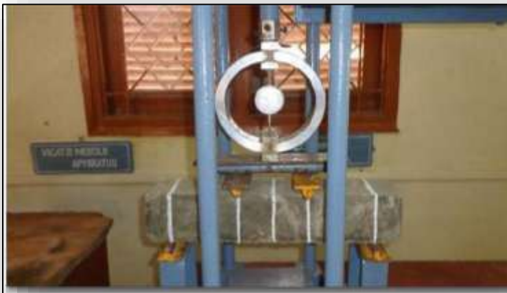
Fig 3. Flexural strength test carried out on specimen in Compression testing machine.
