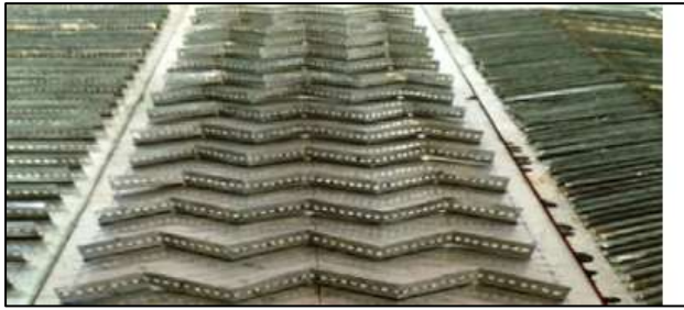
Fig. 20 V perforated baffles[70]
