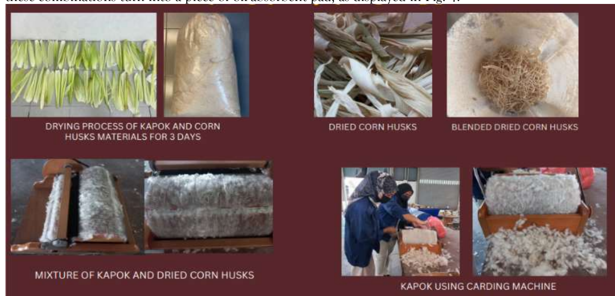
Fig.3 The Carding Process for Kapok and Corn Husks
