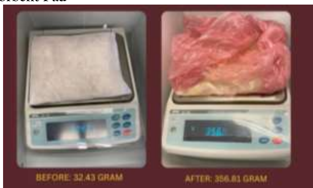
Fig. 4 Kapok and Corn Husks Before and After Oil Spill
