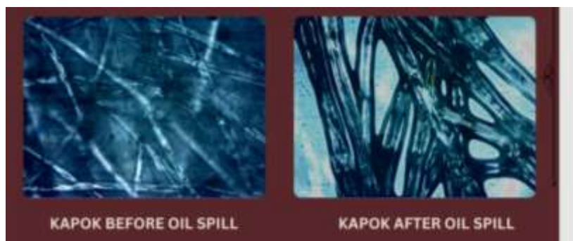
Fig. 6 Lab Result Kapok Image of 10X
