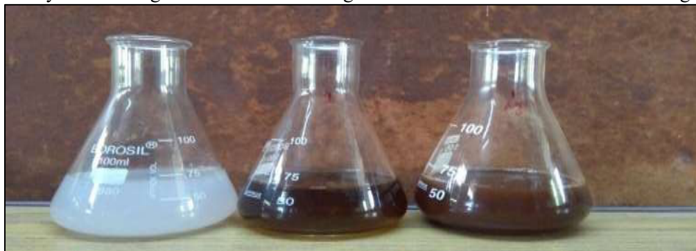
Figure 1: Color change of leaf extracts containing silver nitrate before Acalypha indica .L aqueous leaves extract and after synthesis of silver nanoparticles.
