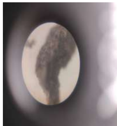
Image 3: Microscopic View of a foreign particle obtained from the Furosemide Sample.
