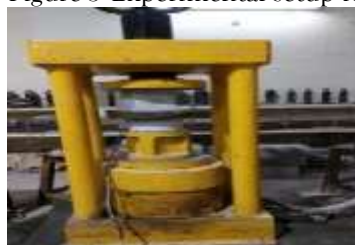
Figure 3 Experimental setup for compression test of cube specimen
