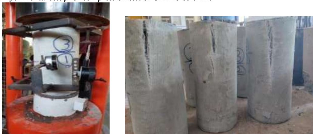
Figure 4 Experimental setup for compression test of CFDTS columns
