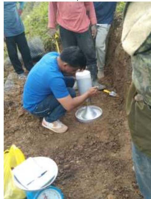
Figure 10. Conduct of FDT on the compacted layers of rice terraces
