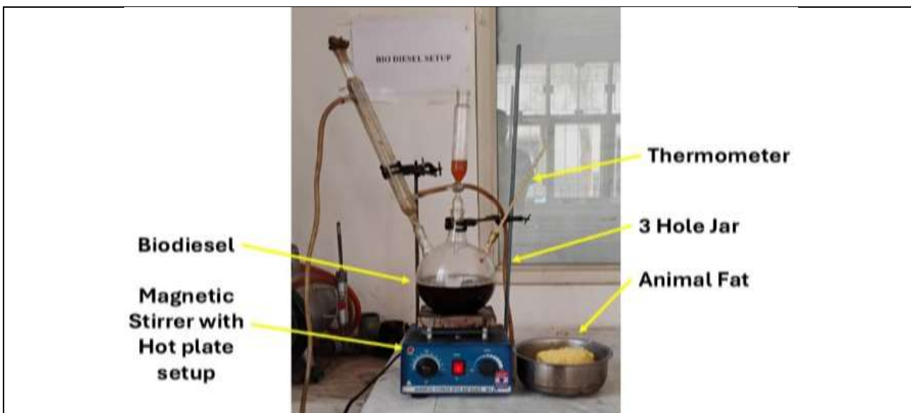
Figure 2 a: Esterification Process setup
