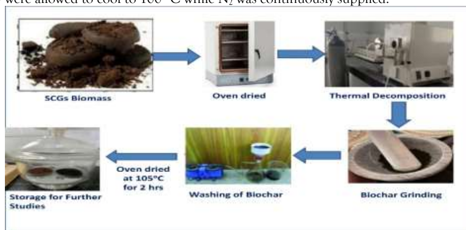
Fig .2 Production Methodology of Biochar derived from SCGs Biomasses
