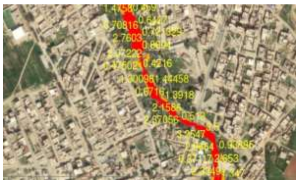
Figure 25: Water Depth Mapping for the Section Passing Through the City Center of Tamazoura
