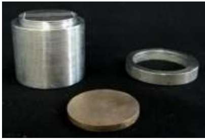
Fig.2 Stainless steel dies standardised
