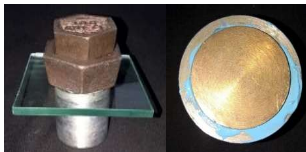
Fig.4 300 grams weight placed while setting of material
