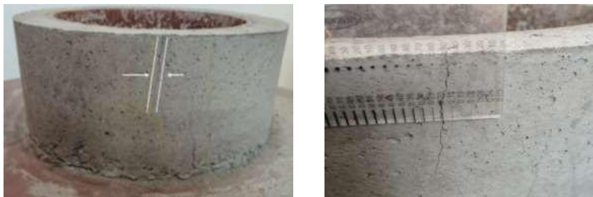
Figure 11 (a): M60 concrete cracking Figure 11 (b): Photo showing crack and crack width measurement
