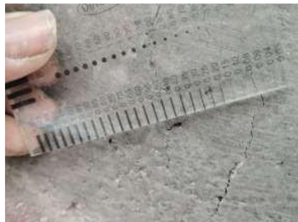
Figure 9 (a): M100 moulded concrete Figure 9 (b): Photo showing of crack and crack width measurement
