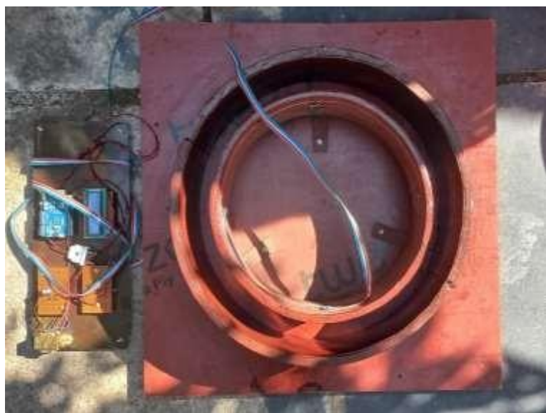
Figure 2: Photograph of ring specimen and data acquisition system
