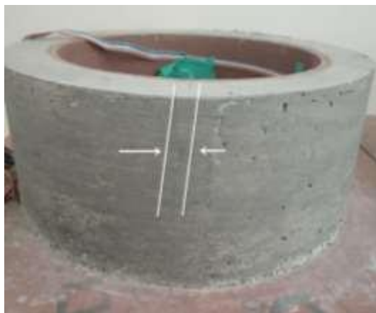
Figure 9 (a): M100 moulded concrete Figure 9 (b): Photo showing of crack and crack width measurement
