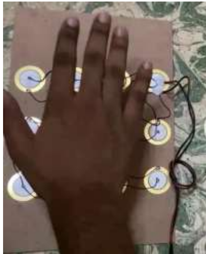
Fig. 6. Application of force on the diaphragm
