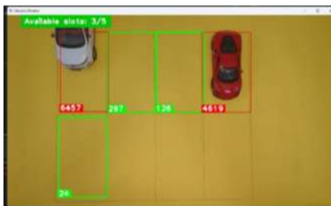
Fig. 8. The change in threshold value of the slot due to the incoming car
