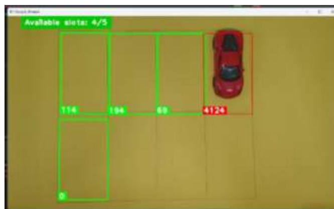
Fig. 7. Available slot count (on the top left), Occupied slots (red bordered), and unoccupied slots (green bordered)
