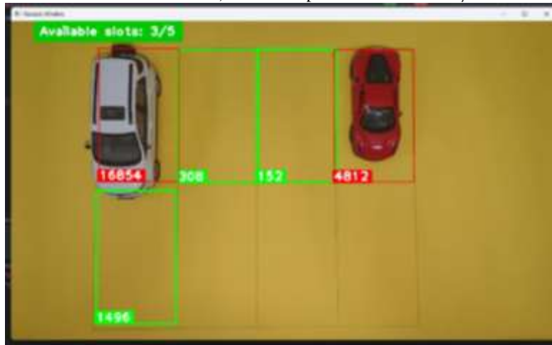
Fig. 9. Final parking position of the new car, resulting in a large threshold value and closing of the slot
