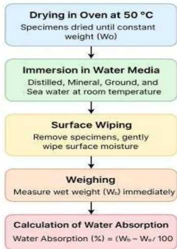
Fig.2: Water Absorption Test Workflow as per ASTM D570
