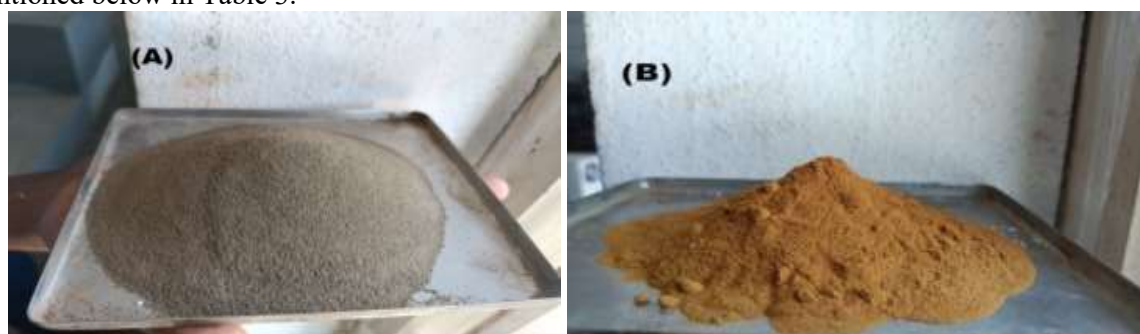
Figure 1: (A) Black cotton soil (B) Calcium lignosulfonate
