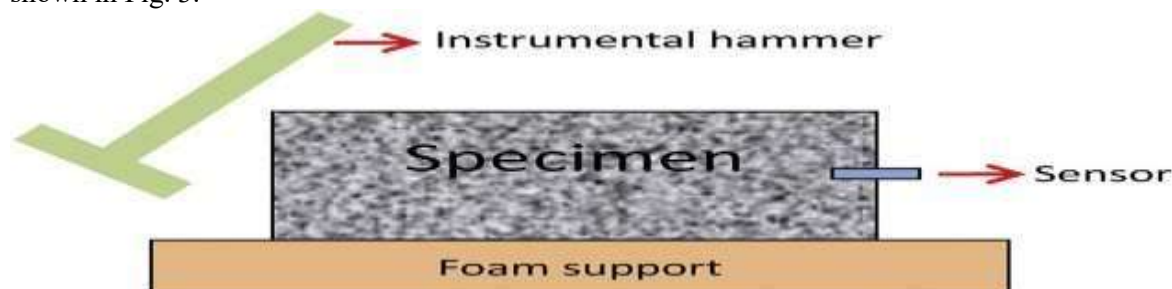
Figure 3. Experimental set-up - Non-linear shock resonance sonic spectroscopy
