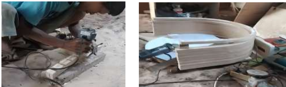
Figure 8. The Process of Forming the Early Chair, by Zaky Ahmad (2024)
