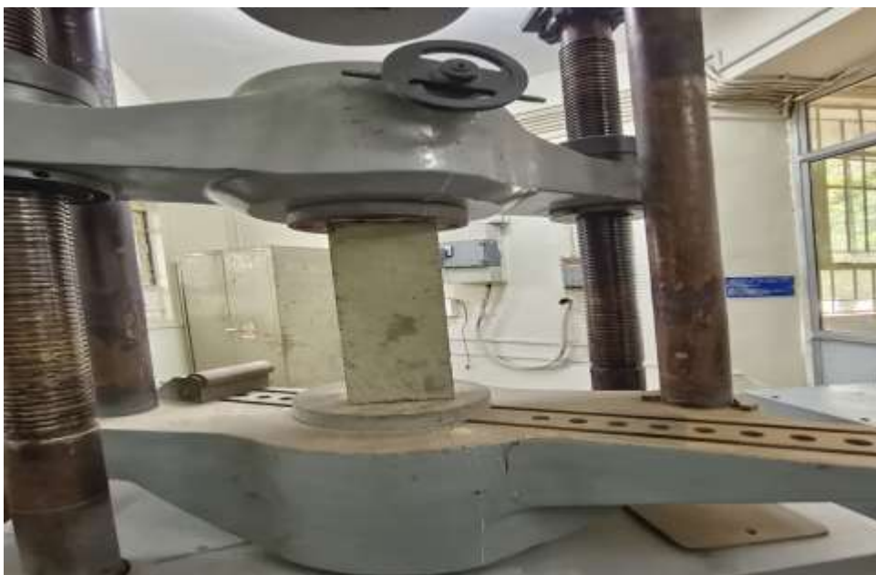
Figure 8. Unwrapped Column specimens
