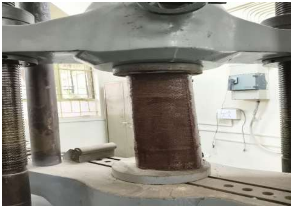
Figure 10. Shape Modified Wrapped Column specimens
