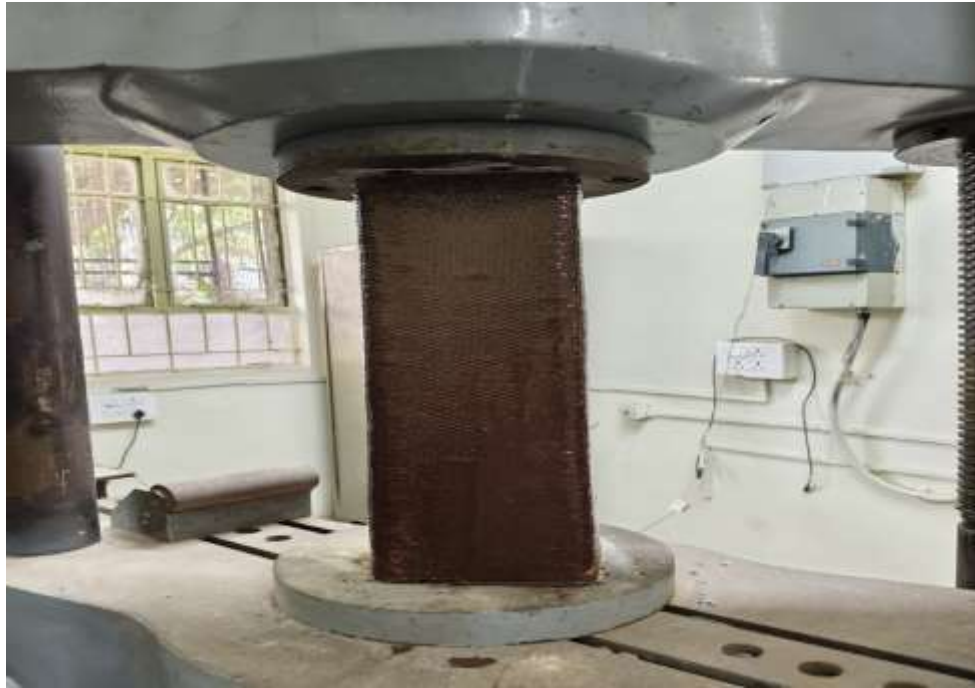
Figure 9. Wrapped Column specimens
