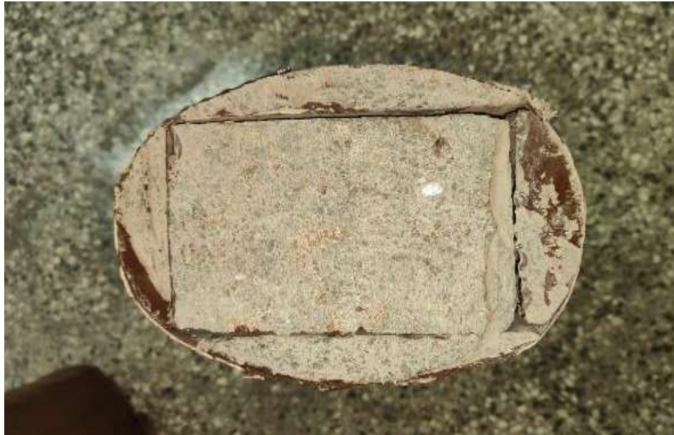
Figure 7. Elliptical GFRP wrapped Column specimens
