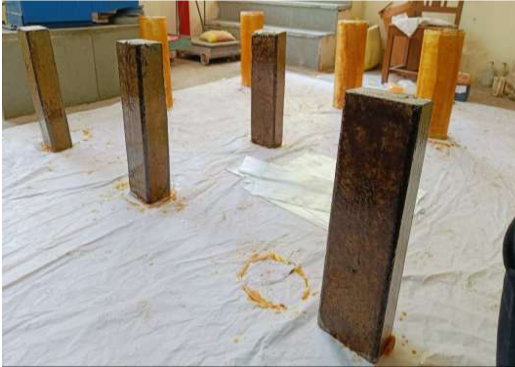
Figure 5. GFRP wrapped Column specimens
