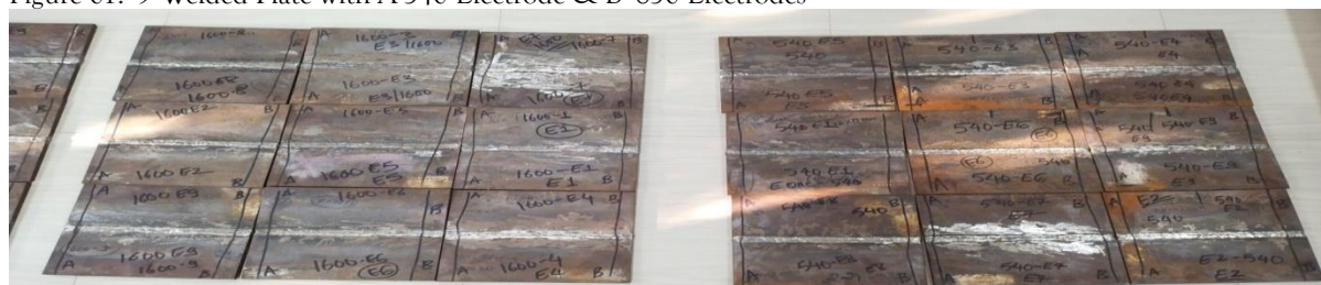
B 1 to B 9 Welded Plate with 850 Electrode
