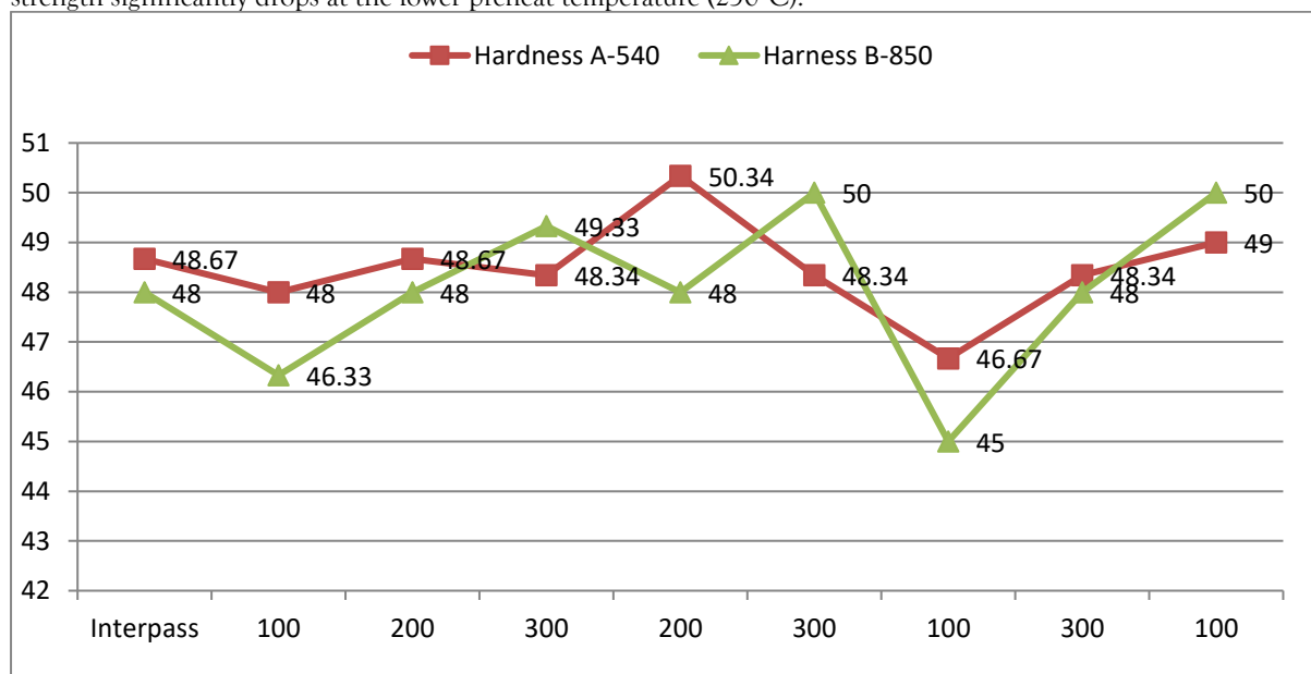
Graph 9:- Interpass Temperature vs Hardness of A 1600 & B 850 Electrodes
