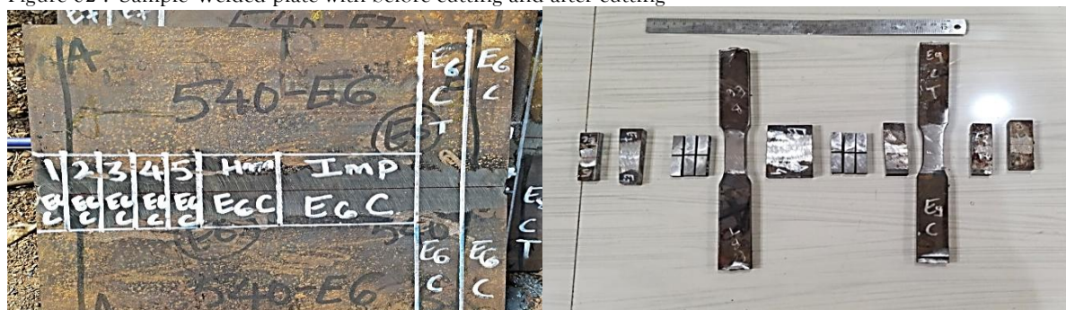
Figure 02 :- Sample Welded plate with before cutting and after cutting
