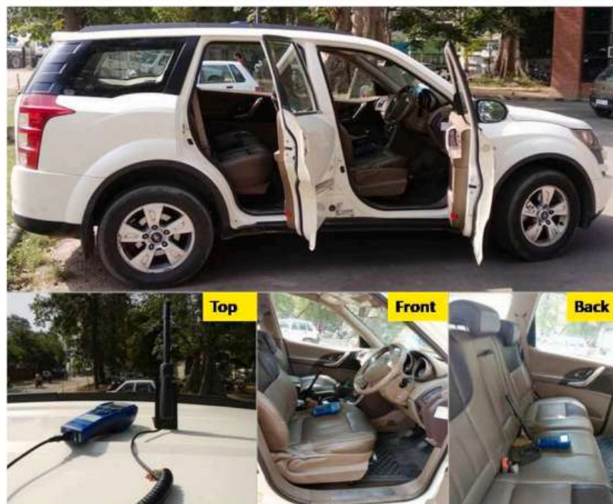
Figure 11: Model car and air quality and meteorological parameter monitoring set-up
